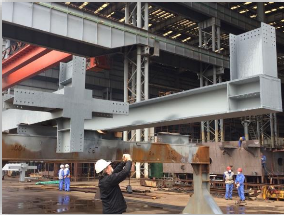
Coal bunkers – 12 huge units of heavy dispensers (63T each) for coal, all fabricated and coated with ZINGA on the Lufeng site.
